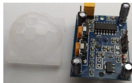
Figure 2.21 PIR sensor - PCB
