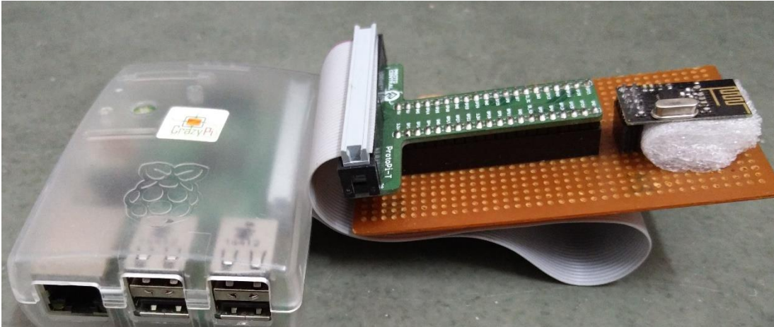
Figure 2.42 Raspberry Pi 2 with nRF24L01+ module
